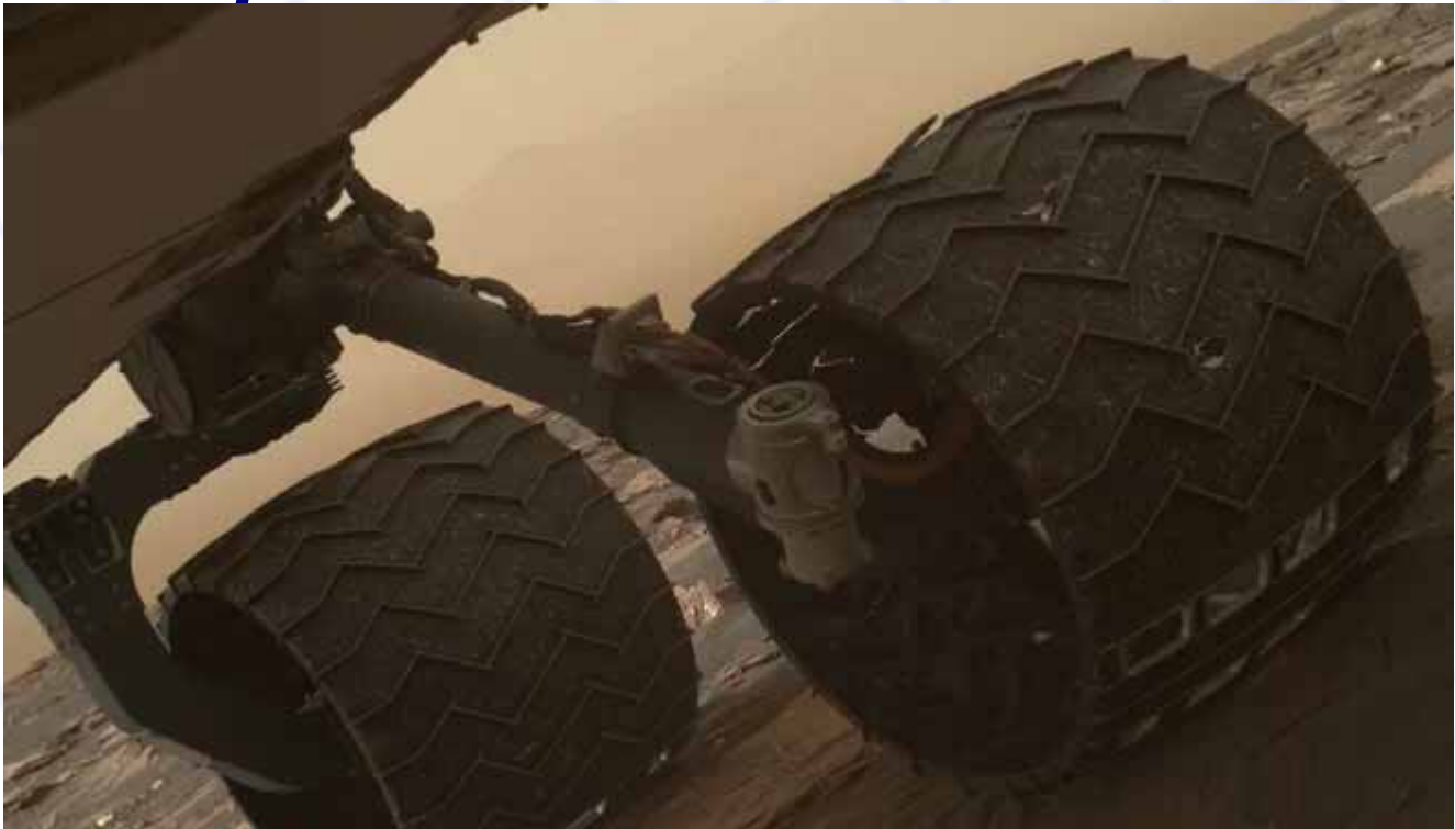
Two of the raised treads on the left middle wheel of NASA's Curiosity rover on Mars suffered breaks in early 2017. One of the breaks is visible as a partially detached section at the top of the wheel, seen here by Curiosity's arm-mounted Mars Hand Lens Imager. Credit: NASA/JPL-Caltech/MSSS
